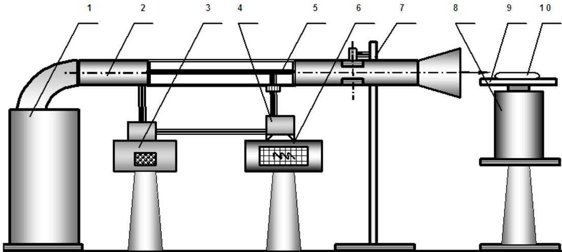
**Figure 1: Experimental Laboratory Equipment for Drying of Low-Fat Milk in a Fixed Position on the Platform (Thin Layer): 1-Turbine; 2-Gas Pipeline; 3-High Voltage Impulse Generator; 4-Transformer for Increase The Voltage; 5- Electrode-Emitter; 6 -Electronic Oscilloscope; 7 - Tripod; 8-Electronic Weighing Device; 9 - Dielectric Platform; 10-Sample of Low-Fat Milk**
